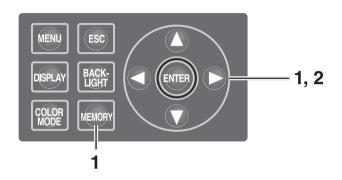
When the power switch is OFF (O), turn it to ON (I) while pressing <u>MEMORY</u> key, key and key simultaneously.
